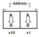
Before communication, you must assign a slave ID to the PROFIBUS slave, If you would like to assign an address between 0 - 99, you need to change the rotary switch to the desired address. If you would like to assign an address which is over 99, you must set it in the MGate utility.
