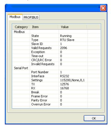
There are two parts. In Modbus tab, the first part is the information regarding Modbus. These details will help you to analyze the Modbus communication.
