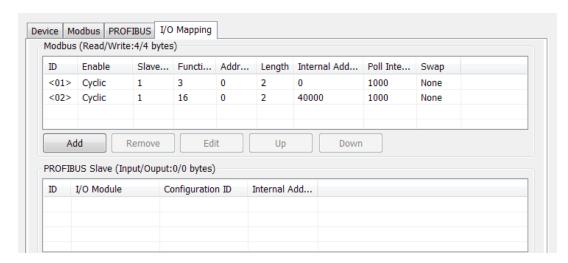
The first command is to read Modbus device's command with function code 03 and the acquired data is to be read by the PROFIBUS master; hence, these data are being placed at Input memory area. Therefore, we set I/O type as *Input*, and with total 4 bytes data length. You may use data length of 2 with *word* data type or use data length of 4 with *Byte* data type.
