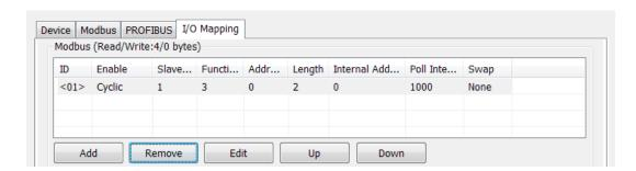
The *I/O Map* function shows the basic I/O mapping relation between Modbus and PROFIBUS. Note that the Modbus related information is marked in <> signs, while PROFIBUS related information is marked in [] signs. The *I/O Map* will show as below figure.
