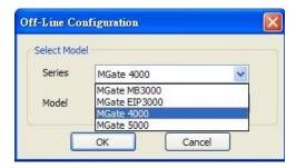
Users can choose "Create new configuration" or "Load existing configuration" to create or modify configurations.
