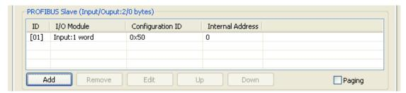
Follow the above steps, you can map all of Modbus requests you need into IO module. In this way, MGate 4101-MB-PBS can communicate between PROFIBUS protocol and Modbus protocol.
