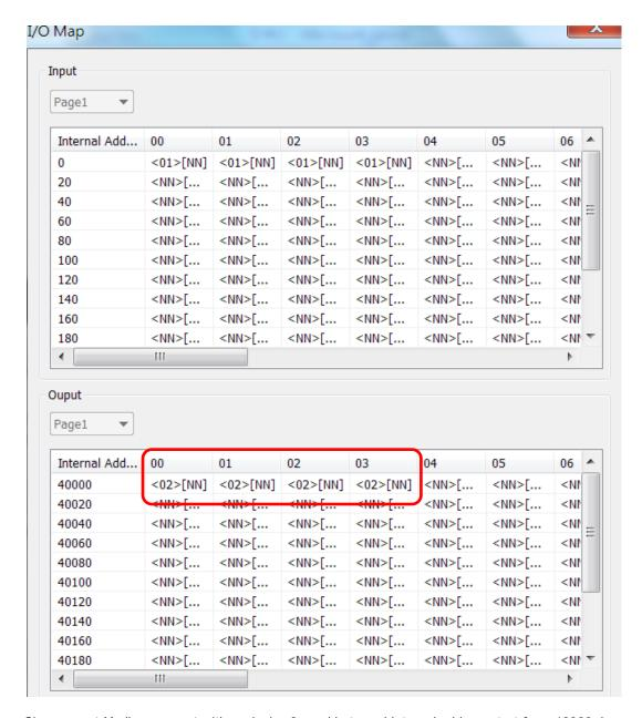
Since we set Modbus request with pack size 2 word byte and internal address start from 40000, hence, the MGate will allocate the first 4 bytes from internal memory address (40000~40003). In summary, the Input or Output memory being allocated is depended on the type of Modbus command (read or write).
