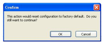
After the MGate Manager resets completely, MGate Manager will automatically execute a Broadcast Search for all MGate units on the LAN and the recording COM port. Your MGate should reappear in the list of units.
