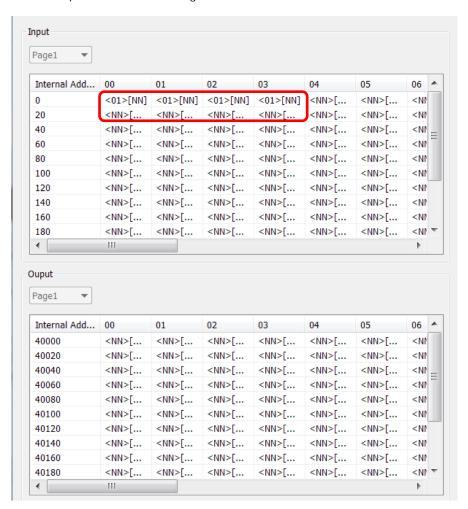
Since we set Modbus request with packet length 2 word byte and internal address start from 0; hence, the MGate will allocate the first 4 bytes from internal memory address (00~03). In other hands, if the Modbus function code 05, 06, 15, and 16 is being chose, that is, write command, the memory it used will be allocated in output memory area. For example, if we adopts function code 16 with packet length 2 (word byte) starting from Internal Address 40000.
