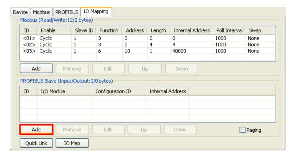
Then, a dialog which is used to set up the IO module will appear, please adjust the parameters which correspond with the Modbus requests you set before. Click **OK** to record this IO module.
