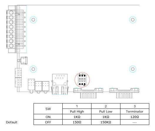
In some critical environments, you may need to add termination resistors to prevent the reflection of serial signals. When using termination resistors, it is important to set the pull high/low resistors correctly so that the electrical signal is not corrupted. The MGate uses jumper settings or DIP switches to set the pull high/low resistor values for each serial port.
